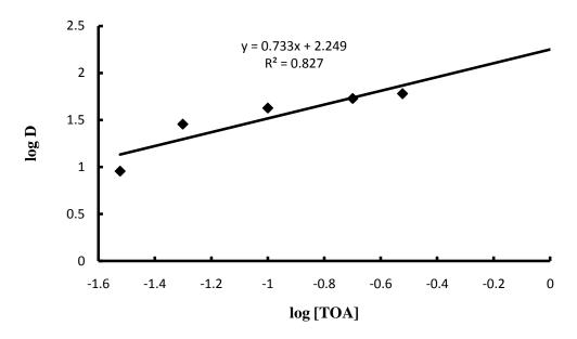
Fig.3.3. Plot of log D versus log [TOA] in the extraction of 0.001M La (III) from 1M HNO<sub>3</sub>.
