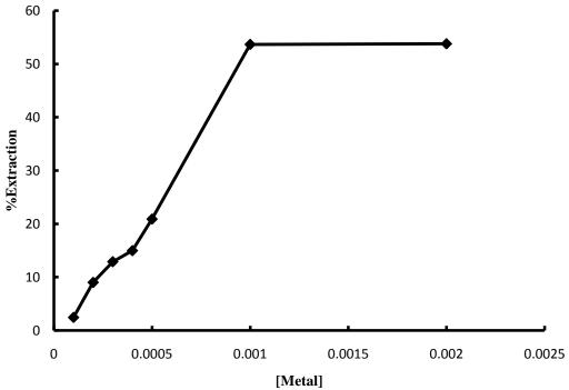
Fig. 3.6.Effect of metal ion concentration for extraction of La(III) from 1M HNO<sub>3</sub> using 0.1M TOA.
