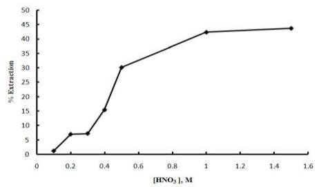
Fig.3.2. Effect of nitric acid concentration on the percentage of extraction of 0.001M La(III) using of 0.1M TOA
