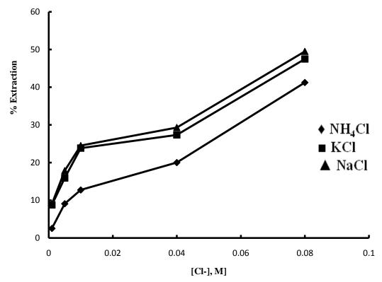
Fig.3.5. Effect of chloride ion concentration on the extraction of 0.001M La (III) from 1M HNO<sub>3</sub> using 0.1M TOA in kerosene.
