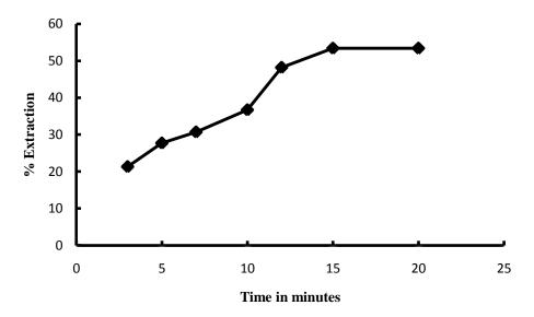
**Fig.3.1.** Plot of % Extraction versus equilibration time in the extraction of 0.001M La(III) from 1M HNO<sub>3</sub> using 0.1M TOA in kerosene.
