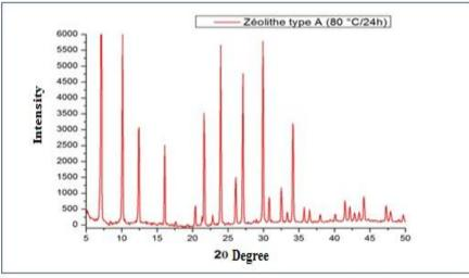
**Fig 8:** XRD of zeolitic type A (T =  $80 \circ C / 24h$ )
