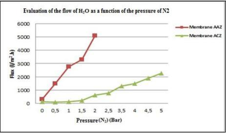
Figure 9: Flow through membranes ACZ and AAZ
