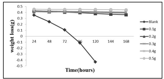
Fig. 2: Variation of Log ( $W_1 - \Delta W$ ) with time for mild steel in 1M H<sub>2</sub>SO<sub>4</sub> at different concentrations of extracts.
