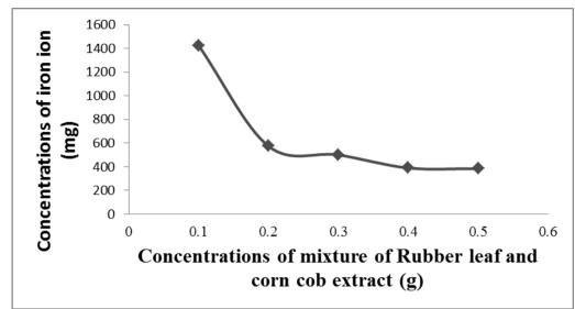
**Fig. 5:** Variations in concentrations of Iron ions ( $Fe^{2+}$ ,  $Fe^{3+}$ ) in 1M H<sub>2</sub>SO<sub>4</sub> acid solution from AAS.
