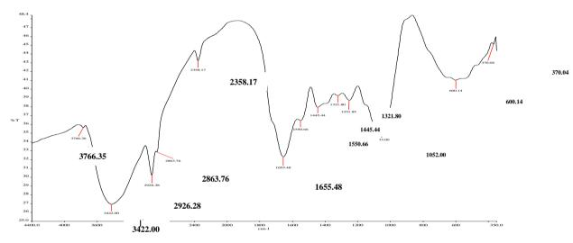
Fig. 6: FTIR Spectrum of Rubber Leaf Extract
