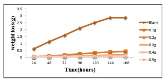
Fig. 1: Variation of weight loss with time for mild steel in 1M H<sub>2</sub>SO<sub>4</sub> at different concentrations of extracts.
