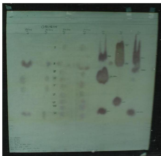
Fig.1: Chromatogram of acetonitrile-water vapour showing formation of amino acids heated up to 100 hrs. under pre biotic wetting drying conditions.
