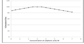
Fig. 2: Extraction behavior of Zinc (II) with synergistic mixture of N-n-octylaniline and Trioctylamine in xylene as a function of concentration of sulphuric acid at 0.25M potassium thiocyanate.
