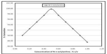
Fig. 4: Extraction behavior of Zinc (II) at fixed concentration of Trioctylamine (TOA) (0.5%), by varying the concentration of N-n-octylaniline.
