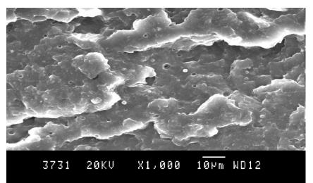
Figure 4a SEM of PA6 + TPU with 3% CLOISITE N
