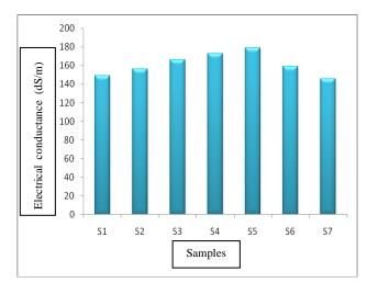
Fig. 4: Electrical conductivity of brine samples during the stages of crystallization
