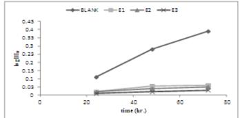
Figure (10): Variation of Log I/Io with oxidation time of lube oil with additives of sulfur ratio = 1.5% with different basicity (E=neutral, E<sub>2</sub>=basic and E<sub>3</sub>=overbasic).
