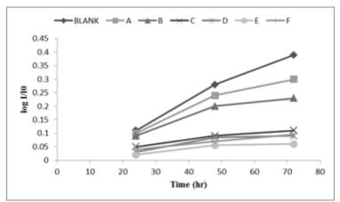
Figure (7): Variation of Log I/Io with oxidation time of lube oil without and with additives (A, B, C, D, E and F).
