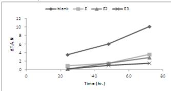
Figure (9): Variation of T.A.N. with oxidation time of lube oil with additives of sulfur ratio = 1.5% with different basicity (E=neutral, E2=basic and E3=overbasic
