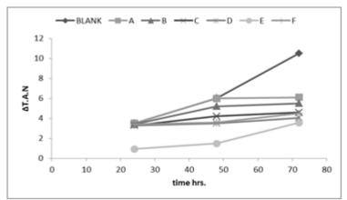
Figure (6): Variation of  $\Delta$ T.A.N. with oxidation time of lube oil without and with additives (A, B, C, D, E and F).
