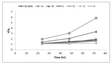
Figure (5): Variation of V/Vo with oxidation time of lube oil without and with additives (A, B, C, D, E and F).
