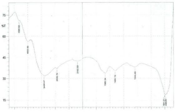
Fig 2: FTIR Spectrum of Modified Soybean Adhesive
