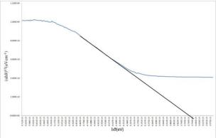
**Fig. 3** Relation between  $(\alpha h \vartheta)^{1/2}$  and  $h \vartheta$  for the polyaniline
