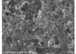
Fig. 5 SEM image of Polyaniline
