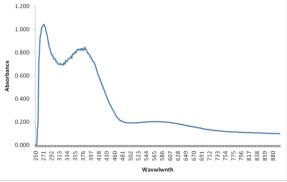
Fig 2 UV-Visible spectrum of Polyaniline
