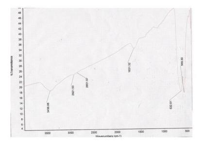
Figure 2: IR Spectra of the synthesized chromium oxide nanoparticles
