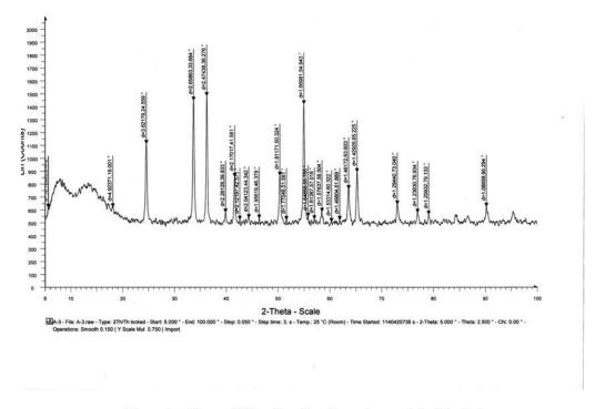
Figure1: X-ray diffraction for chromium oxide (Cr<sub>2</sub>O<sub>3</sub>)
