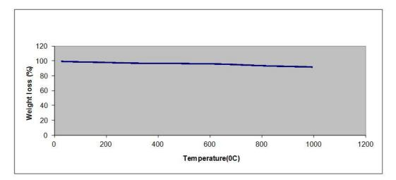
Figure 3: TGA Graph of chromium oxide NPs
