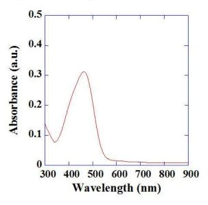
Figure 4: UV-Visible Spectra of the chromium oxide
