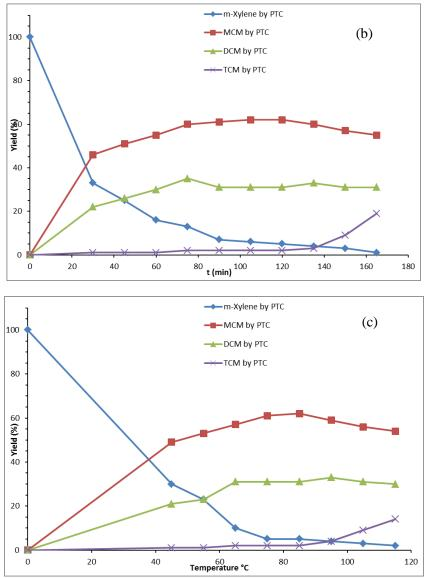
Figure (1): Influence of (a) molar ratio [CH<sub>2</sub>O/m-xylene], (b) reaction time and (c) temperature on the chloromethylation.
