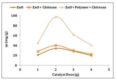
**Figure 5:** Effect of varying dosage on the adsorption of methylene blue. Experimental Condition: Mass of catalyst 0.25 - 1.0g, contact time 90 mins at pH 6.
