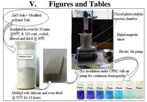
Figure 1: Illustration demonstration the formation of catalyst and its application in the adsorption of Methylene blue dye.
