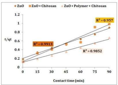
**Figure 6:** Pseudo-second-order kinetics plot for MB dye onto polymer coated ZnO with chitosan, ZnO with Chitosan and ZnO. Experimental Condition: MB dye concentration = 50 ppm, Mass of catalyst = 0.5 g, contact time = 90 mins at pH 6.
