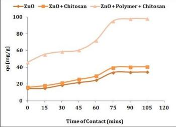
**Figure 4:** Effect of contact time on the adsorption of methylene blue. Experimental Condition: Mass of catalyst =0.5g, contact time 0-105 mins at pH 6.
