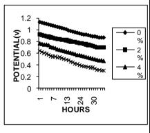
Fig 6: Open circuit potential test in 3.5 % sodium chlorides solution
