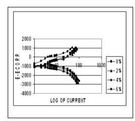
Fig 7: Ptentiostat test in 0.035 % sodium chlorides solution
