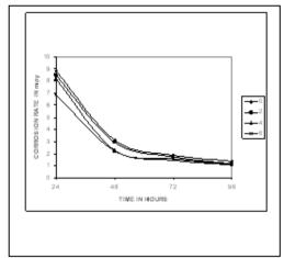
Fig.3: Weight loss corrosion in 3.5% sodium chloride solution
