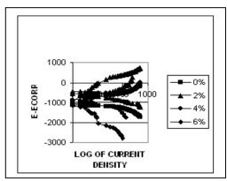
Fig 9: Potentiostat test in 3.5 % sodium chlorides solution
