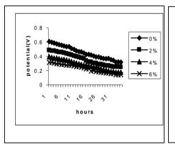
Fig 5: Open circuit potential test in 0.35 % sodium chlorides solution
