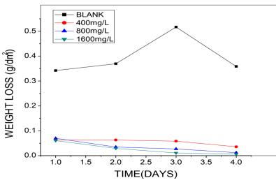
Fig 1 : Weight loss against time for mild steel in 0.5 M  $H_2SO_4$  in the absence and presence of 400 mg/L, 800 mg/L and 1600 mg/L of water extract of SM leaves.
