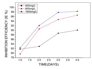
Fig 2: Inhibition efficiency against time for mild steel in 0.5 M  $H_2SO_4$  containing 400 mg/L, 800 mg/L and 1600 mg/L of water extract of SM leaves.
