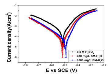
Fig 3 Potentiodynamic polarization curves for mild steel in 0.5 M  $H_2SO_4$  in the absence and presence of 400mg/L and 1600mg/L SM- water extract.
