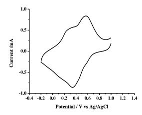
Fig 2: Cyclic voltermmetry for surface PANI modified electrode in 0.5 mM  $H_2SO_4$  at scan rate 100 mVs<sup>-1</sup> between potentials of -0.4 and 1.4 V.
