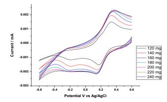
Fig 3: Cyclic Voltammogram of Effect of concentration of PANI in 0.1M K<sub>3</sub>Fe(CN)<sub>6</sub> in a 1M supporting electrolyte of KNO<sub>3</sub> at PANI CPEs at a scan rate of 20 mVs<sup>-1</sup>
