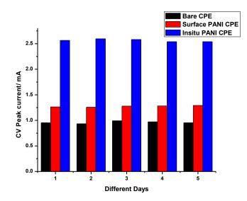
Fig 6: Repeatability study of the bare, Surface and Insitu PANI modified CPE towards 0.1M K<sub>3</sub>Fe(CN)<sub>6</sub> in a 1M supporting electrolyte of KNO<sub>3</sub>
