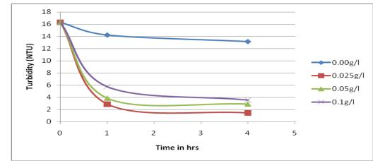
Figure 5. Optimal M. oleifera dosage for synthetic turbid water at 16.3 NTU initial turbidity
