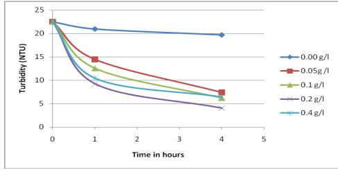
Figure 6. M. oleifera optimal dosage for naturally turbid water
