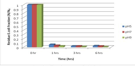
Figure 9. Effect of pH on E. coli disinfection
