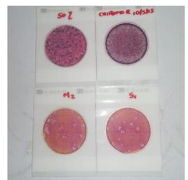
Figure 2. Pictorial presentation of the E. coli results after filtration.
