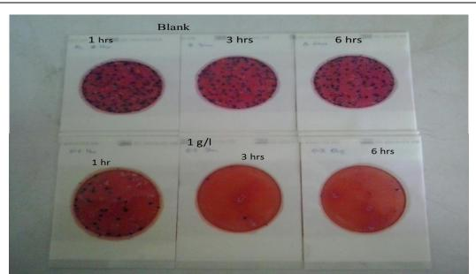
Figure 8. Pictorial illustration of the effect of time for the blank and 1g/l dosages after 1, 3 and 6 hours of coagulation.
