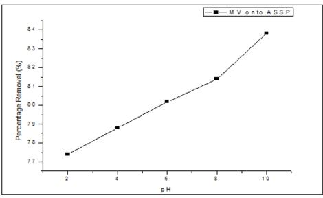
Fig.13: Effect of pH on the percentage removal of MV onto ASSP
