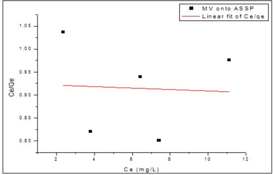
Fig.14: Langmuir isotherm plot for the adsorption of MV onto ASSP
