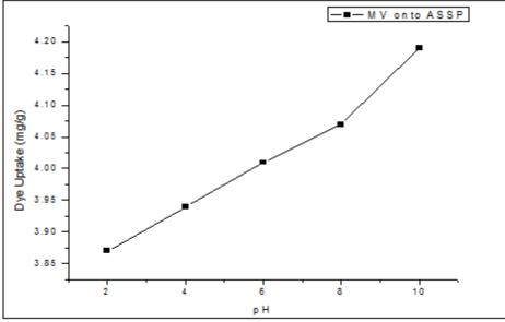
Fig.12: Effect of pH on the adsorption capacity of MV onto ASSP
