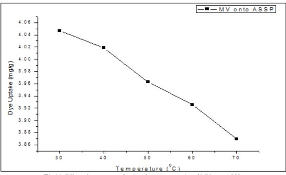
Fig.11: Effect of temperature for the adsorption capacity of MV onto ASSP
