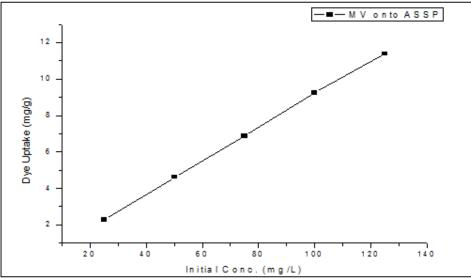
Fig.8: Effect of initial concentration for the adsorption capacity of MV onto ASSP
