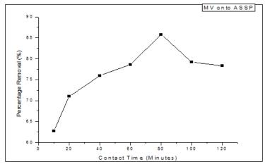
Fig.5: Effect of contact time for the percentage removal of MV onto ASSP
