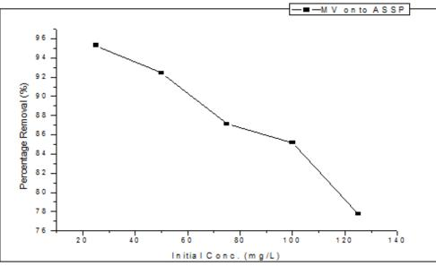
Fig.9: Effect of initial concentration for the percentage removal of MV onto ASSP
