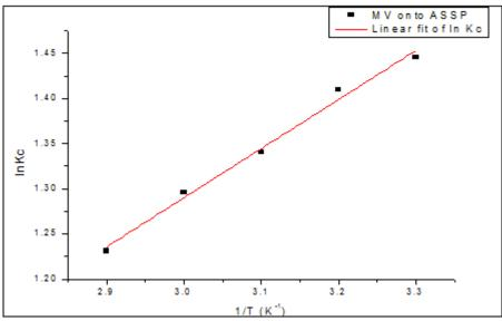
Fig.18: Van't Hoff plot for the adsorption of MV onto ASSP
