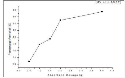
Fig.6: Effect of adsorbent dosage for the percentage removal of MV onto ASSP
