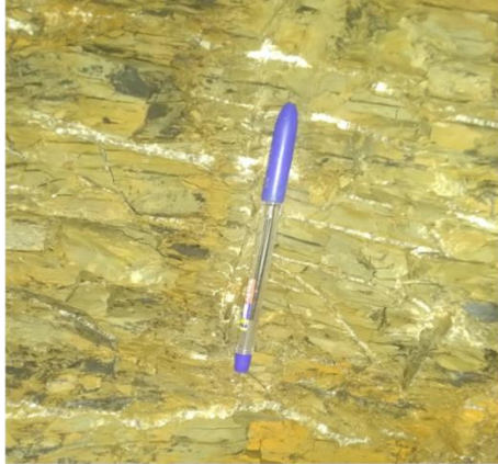
Plate I: Gypsum occurring concordantly within the shale
