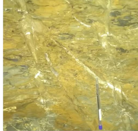
Plate II: Gypsum beds crosscutting the shale
