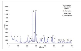
Figure (2) Representative XRD Chart for Special Diffraction Pattern of the Minerals in soil
