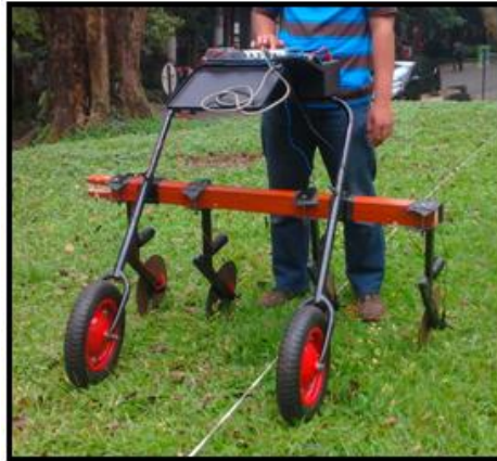
Fig.3. Disk electrode device of electrical resistivity
