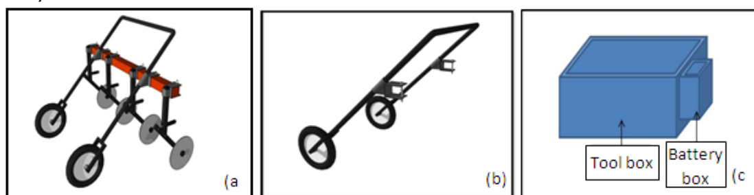
Fig.2. (a) Disk electrode design of electrical resistivity (b) Design wheel sets that will be applied to the disk electrode (c) The design of the tool box as a container resistivity meter and battery.
