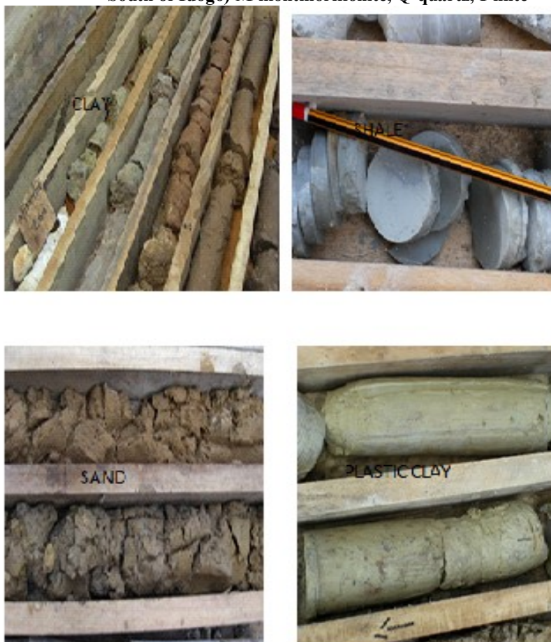
Plate 1-4: X-lithological samples of marl, shale, sand and clayey-shale sediments from the study area
