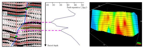
a. Buried depth -Fault separation diagram b. Fault separation distribution contour map Figure.1 Analysis of well seismic data and break distance of break point
