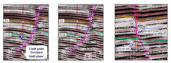
a. Well seismic calibration error b. Corrected well seismic correspondence c. Deviation data error and fault plane does not match the breakpoint
