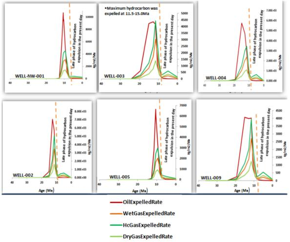
**Figure 5:** Main charge is predicted to have Maximum hydrocarbon expelled from the source rock at 11.5-15.0Ma and a later phase at 8Ma – present day with oil expelled rate at almost zero.
