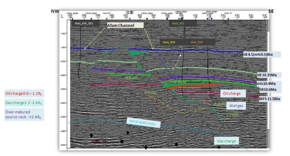
Figure 6: Diagram showing the generation, accumulation and migration of the hydrocarbon charge in the study area.
