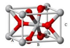
Figure 3. The model of the unit cell of the crystal rutile SnO<sub>2</sub>
