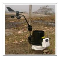
Fig 1.3: The Integrated Sensor Suit (ISS) on site at Awka
