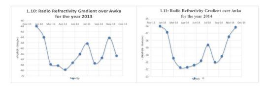
Fig 1.10 and 1.11 shows Radio Refractivity Gradient over Awka for the year 2013 and 2014 respectively. The average monthly refractivity gradient dN/dh from 2013 to 2014 over Awka was calculated and found to vary from -55.97 N – units/m to -68.07 N – units/m for the dry season periods and -57.44 N – units/m to -68.81 N – units/m for the wet season periods.
