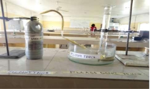
Figure 2: Experimental Set-Up For Biogas Production
