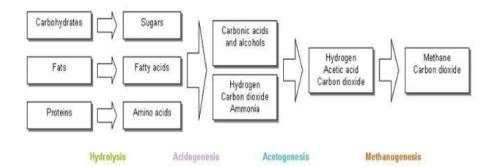
Figure 1: Stages Of Biogas Production(Kozani,2014).
