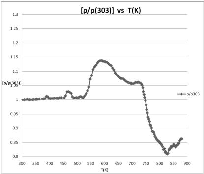
Figure 2: Resistivity Ratio,  $\rho/\rho_{(303)}$  versus Temperature (T) of amorphous Fe<sub>78</sub>Ce<sub>2</sub>B<sub>20</sub> alloy
