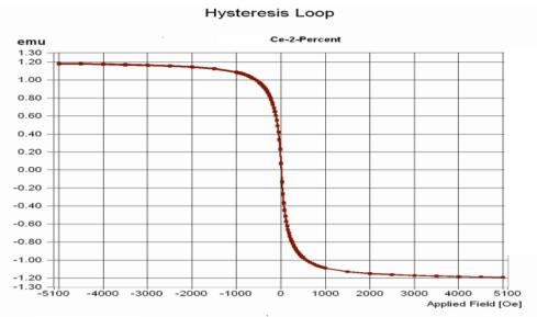
Figure 1 The Hysteresis curve of amorphous Fe<sub>78</sub>Ce<sub>2</sub>B<sub>20</sub> alloy
