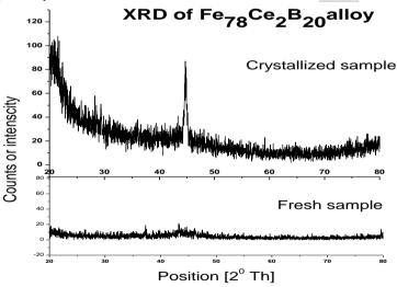
Figure 3 XRD pattern of amorphous and crystallized Fe<sub>78</sub>Ce<sub>2</sub>B<sub>20</sub> alloy recorded at room temperature.
