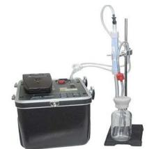
Fig 2: Arrangement of apparatus for measuring radon content in the carbonated drinks.
