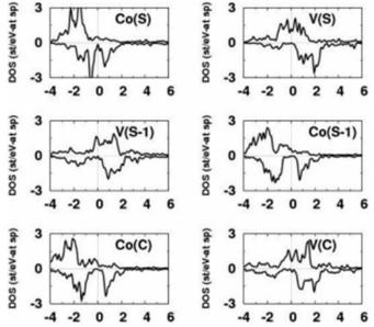
**Fig. 2** Atom-projected spin-polarized density of states (DOS) for the chosen atoms of the Co- (left-pannels) and V-terminated (rightphannels) CoV(001) surface. The spin-down DOS values are multiplied by a negative number, and the Fermi levels are set to zero.
