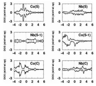
**Fig. 3** Atom-projected spin-polarized density of states (DOS) for the chosen atoms of the Co- (left-pannels) and Nb-terminated (rightpannels) CoNb(001) surface. The spin-down DOS values are multiplied by a negative number, and the Fermi levels are set to zero.
