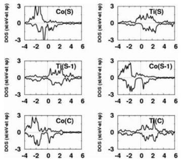
Fig. 1 Atom-projected spin-polarized density of states (DOS) for the chosen atoms of the Co- (left-pannels) and Ti-terminated (rightpannels) CoTi(001) surface. The spin-down DOS values are multiplied by a negative number, and the Fermi levels are set to zero.
