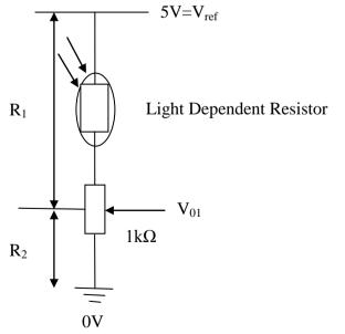
Figure 3.1.1: Light Intensity Circuit
