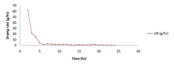
Figure 4.5: Drying rate with time of sliced Yam in the open sun
