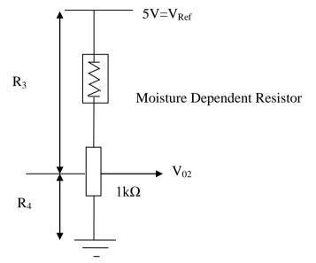
Figure 3.1.2: Moisture Content Measurement Circuit
