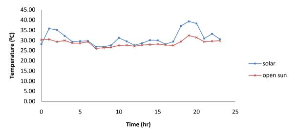
Figure 4.1: Variation of temperature of sliced Yam in the solar concentrator dryer and open sun
