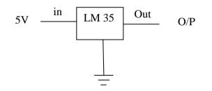
Figure 3.1.3: Temperature Circuit
