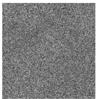
Figure 2. a gamma camera image for phantom that generated by ink jet printer for uniformity test
