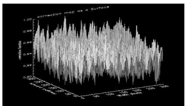
Figure 4. shade-surface of the correction matrix that used to overcome the problem of uniformity if the value of uniformity exceeds the limits.
