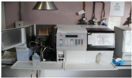
Fig. 1: Atomic Absorption Spectrophotometer Set-Up
