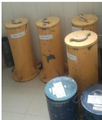
Figure 7: Lead Container for Preservation wastages
