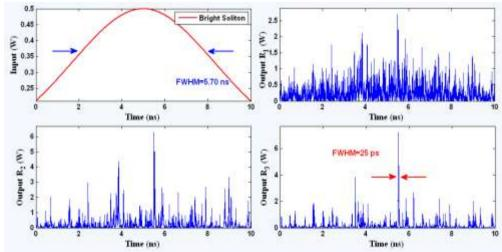
**Fig. 3:** Results obtained when temporal soliton with FWHM=25 ps is localized within a microring device
