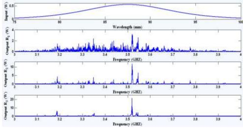
Fig. 2: Results obtained when frequency soliton pulse is localized within a microring device with 20,000 roundtrips, the ring radii are  $R_1$ = 10  $\mu$ m,  $R_2$ = 10  $\mu$ m,  $R_3$ = 12  $\mu$ m
