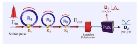
**Fig.1:** Schematic diagram of a continuous variable quantum key distribution with the different time slot entangled photon encoding. PBS, polarizing beam splitter, Ds, detectors, Rs, ring radii and  $\kappa$ s, coupling coefficients.
