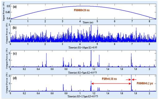
Fig. 2: Results obtained when temporal soliton is localized within a microring device with 40,000 roundtrips where (a): Input bright soliton, (b): Output signal from  $R_1$ , (c): Output signal from  $R_2$ , (d): Output signal from  $R_3$  with FWHM and FSR of 0.2 ps and 0.58 ns respectively
