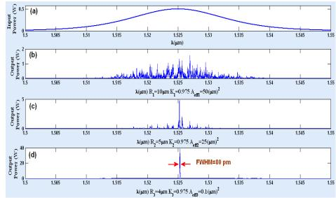
**Fig.3:** Results obtained when a spatial soliton is localized within a microring device with 40,000 roundtrips, where (a): input bright soliton, (b): output signal from  $R_1$ , (c): output signal from  $R_2$ , (d): output signal from  $R_3$  with FWHM of 80 pm
