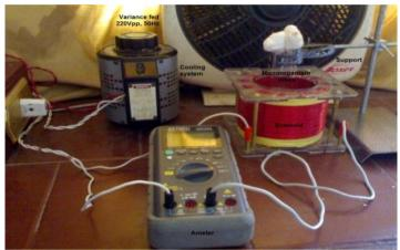
Fig. (1a): The electromagnetic field exposure system.
