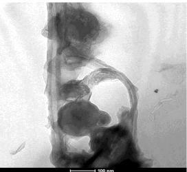
Figure 3 TEM image of Al-CNT composite with 1.5wt% of CNT
