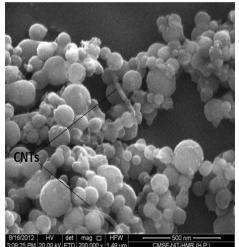
Figure 2SEM image of Al-CNT composite with 2wt% of CNT
