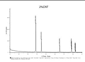
Figure 5 XRD analysis of Al-CNT composite with 2wt% of CNT
