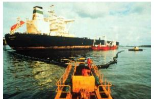
Figure 2.0: Oil booms used to contain oil spill from an oil tanker.
