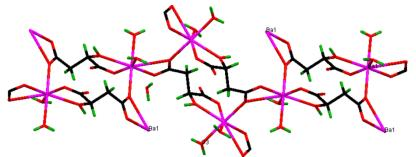
Figure 3. Polymeric structure of barium malate trihydrate
