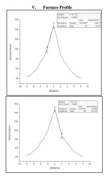
Temperature gradient is 24°C/cm on one solid-liquid interface and 30°C/cm at the other interface. Molten-Zone length was 4-5 mm.
