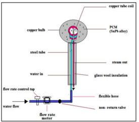
Figure 4: Components of the compensating absorber
