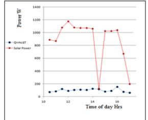
Figure 9: Performance of Non-Compensated Absorber
