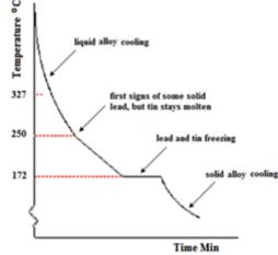
Figure 2: Cooling curve of 60Sn40Pb alloy [Source -www.chemguide.co.uk]
