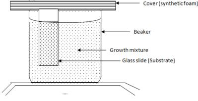
Fig. 1. Experimental set up.
