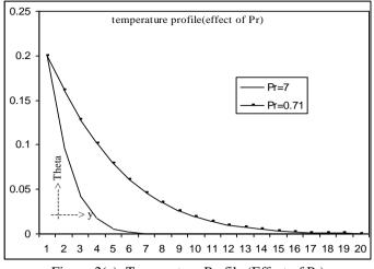
Figure-2(a): Temperature Profile (Effect of Pr)
