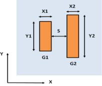
Fig.1 Geometry of the gold rods on glass substrate
