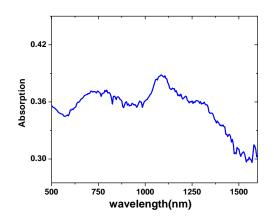
Fig.3.Measured experimental absorption spectra for the gold rods. Two absorption peaks can be observed indicating of the resonances at wavelengths of 781.2 nm with a peak of 37% and 1083.3nm with a peak of 39% respectively.
