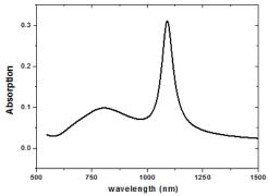
Fig.2 Absorption of the gold rods. Two absorption peaks can be observed at the resonance wavelengths of 803.6nm with peak of 10% and 1089.3nm with a peak of 31% respectively.
