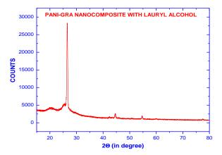
Fig.5: XRD of PANI-GRA nanocomposite treated with lauryl alcohol.
