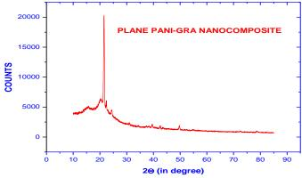
Fig.4:XRD of plane PANI-GRA nanocomposite
