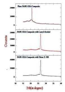
Fig. 6: Combined XRD of three nanocomposites shows peak shift towards higher value of  $2\theta$
