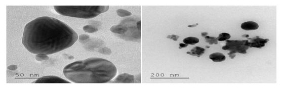
Fig.5.TEM image of synthesized silver nanoparticles using leaf extracts of Ipomoea staphylina.
