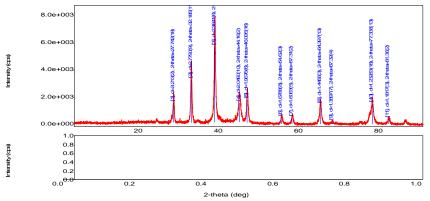
Fig.4. XRD spectrum of synthesized silver nanoparticles using leaf extracts Ipomoea staphylina.
