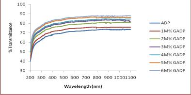
Fig.4. UV- Spectrum of conventionally grown pure and Glycine doped ADP (GADP) crystals with different concentrations
