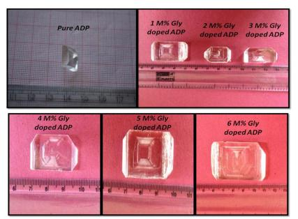
Fig.1. Photographs of pure and Glycine doped ADP (GADP) crystals with different concentration (1 mole% to 6 mole%)
