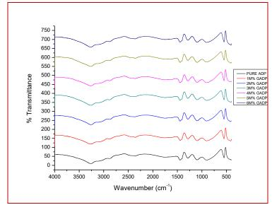
Fig.3. FTIR spectrum of pure and Glycine doped ADP (GADP) crystal
