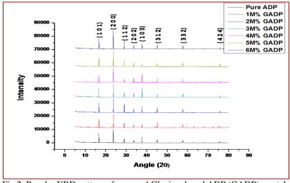
Fig.2. Powder XRD pattern of pure and Glycine doped ADP (GADP) crystals
