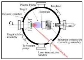
Fig. 1 Schematic diagram of Experimental Setup
