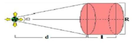
Fig.1 Representation the experimental setup. [(S) the point source, (d) source- detector distance, (l) detector length and (R) the detector diameter].
